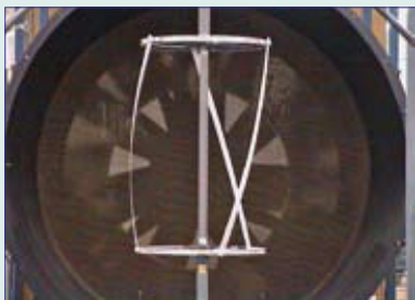
The first prototype Turby in front of the wind tunnel of the Wind Energy section at TU Delft's Stevin Laboratory. It has racing bike wheels fitted with aerodynamic spokes at its top and bottom. The manufacturer of the first prototype thought the aerodynamic spokes would keep the drag figure down. However, the model disintegrated because the bolt used to secure the position of the two wheels broke
